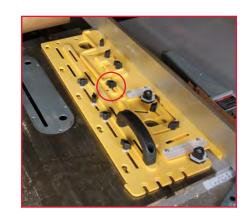
2. For the steeper taper, set up the MEMORYLOCK Stop in the angled slot towards the rear of the jig. Again adjust the stop so the two nubs touch the edge of the movable part of the jig. With the stops set, you can switch between them by simply loosening the locking knob and pivoting the bottom plate.
