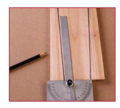
4. The black lines and numbers are for the 1/4° and 3/4° (.25° and .75°) settings, and the yellow lines and numbers are for the 3/8° and 7/8° (.375° and .875°) settings. Here the jig is set for 3 1/4°.
