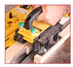
**SAFETY ALERT!** When making a second cut on a tapered piece, the trailing end of the leg will be thinner than the leading end. Make sure the blade isn't set so high that it will cut into the underside of the GRR-RIPPER at the end of the cut. Move the GRR-RIPPER forward if necessary.
