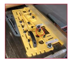
The MICRODIAL Tapering Jig may be used as a large pushblock to straighten the edge of crooked boards on your tablesaw. Attach the Trailing Block and shift the jig's Top Plate to the Jointing Slots. The MICRODIAL Tapering Jig can straighten the edges of boards up to approximately 12" wide and 30" long.
