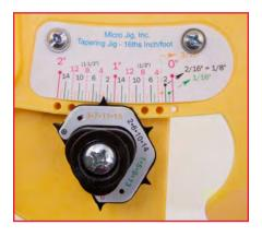
5. For tapers that don't work out to even sixteenth inch increments, use the pointer marked with a black X inside a circle. There is no pin associated with this pointer, so the jig will pivot freely. Here the jig is set to cut a taper just under 1 1/4"per foot.
