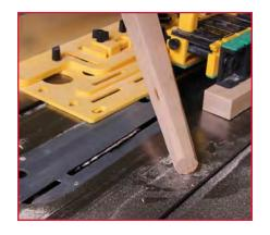
The MEMORYLOCK system allows for quickly shifting between two preset tapers for repeatable cutting. Use the two MEMORYLOCK Stops to memorize two individual tapers.
