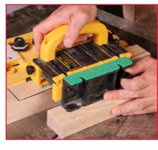
Tighten the knobs to ensure the GRR-RIPPER has good traction.
