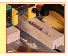
If your project calls for a piece that is tapered equally on opposite sides, you will need to reset your MICRODIAL Tapering Jig in between the cuts. After you make the first cut, you have changed the reference surface for the second cut. Reset the jig by doubling the initial setting as shown in the photos below. Note: On wider workpieces, you can use the tapering jig without GRR-RIPPERs.
