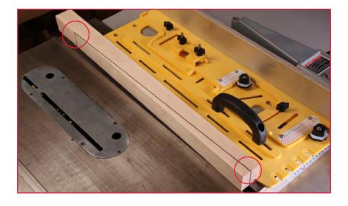
1. Lay out the taper on your workpiece. Hold the piece on your saw so the beginning and end points align with the edge of the miter gauge slot (which should be parallel to the blade). Hold the jig against the rip fence
