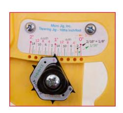
3. To set the jig for the 1/8" inch divisions (1/8", 3/8", 5/8", 7/8"), align the pointer near the black numbers with the appropriate black line on the scale. Here the jig is set to cut a taper of 1 1/8" per foot.
